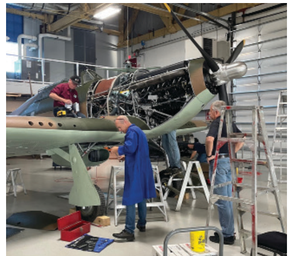
Calgary Mosquito Society working on the Merlin Engine of Hawker Hurricane #5389
