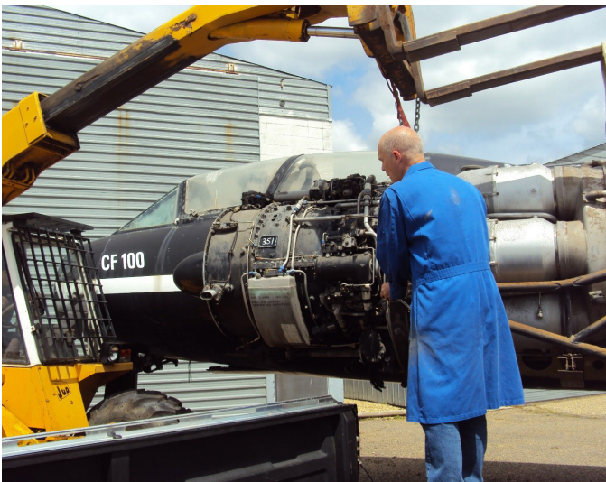
Removal and inspection of Orenda Engine, July 2020
